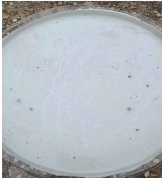
Mixing: It will get hard to stir so you may want to have someone help take turns stirring the cement with you. After you pour the cement into the molds you are supposed to tap them on the ground 2-3 minutes to get the bubbles to rise to the surface.
